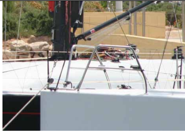
Picture 1 – Custom Boats 1 (Issue: upper rail at deck level)
